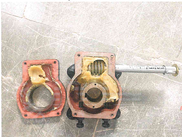
Picture2: No ingress of powder & water observed
